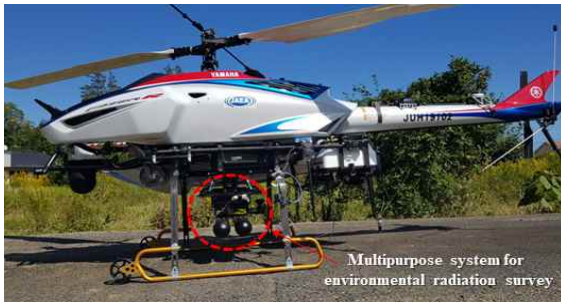
Fig. 8 Unmanned Helicopter with a MSERS
