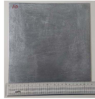
Fig. 2. The manufactured B_4C/Al6061 AMCs by stir casting followed by hot rolling process
