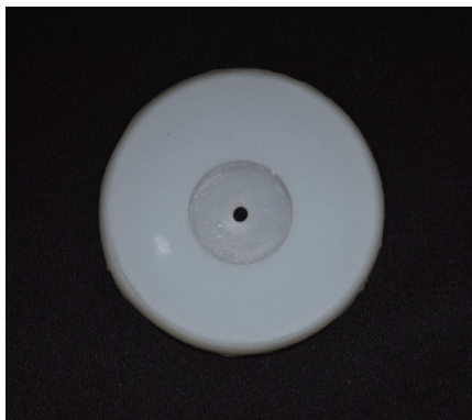
Fig. 2. Silicone mold for bonding conventional resins.
