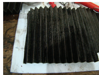
Fig 4. Blockage by engine filter mesh.
