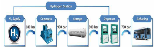
Fig. 1. A diagram of H 2 charging station
