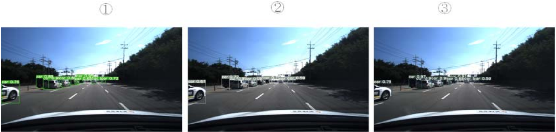
<Fig. 10> Detection results of a KODAS example image with the yolo v3 models trained in 3 datasets on Experiment no.2
