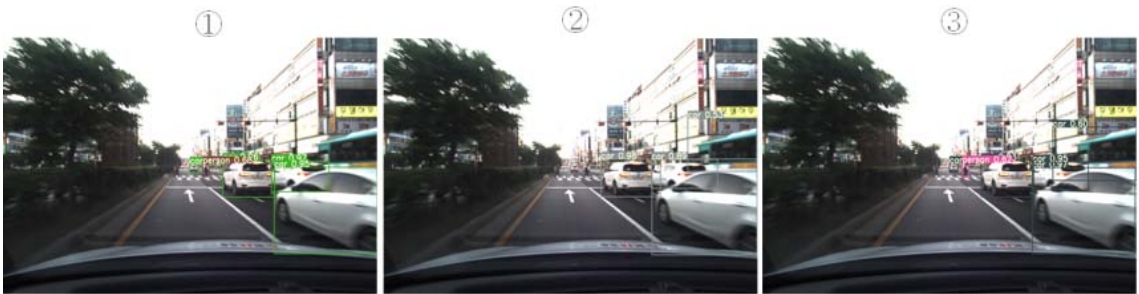
<Fig. 12> Object unrecognized case due to the minimum pixel setting of the virtual environment dataset
