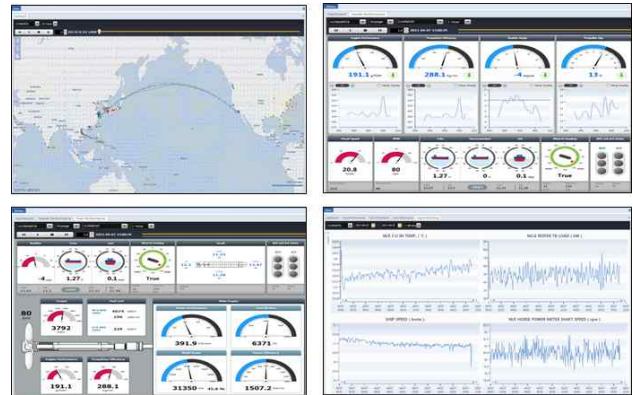
Fig. 7 Photographs of energy efficiency monitoring system (EEMS)
