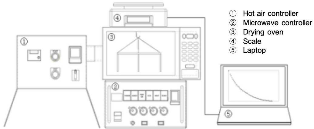
Fig. 2. Microwave - hot air combination drying system.
