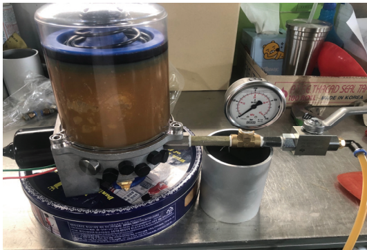
Fig. 2 Experimental test-bed compact automatic lubrication system
