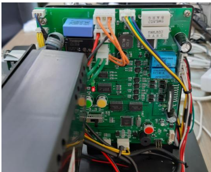
Fig. 4. Control board of multi-dimensional flatbed printer
