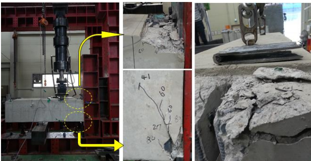
Figure 17. Situation of final failure
