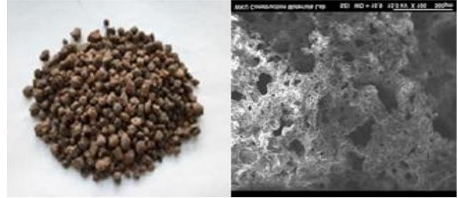
Figure 2. Shape and SEM image of lightweight aggregate
