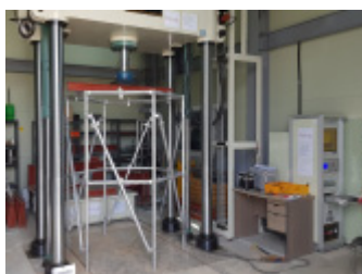
[Figure 7] Bending test for horizontal member
