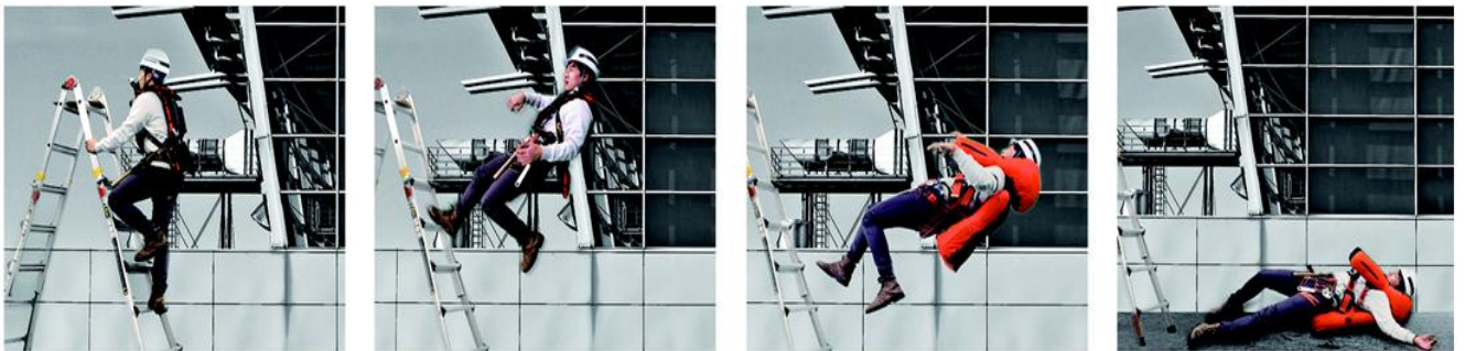
(c) Air cushion deployment sequence in a fall situation during work
