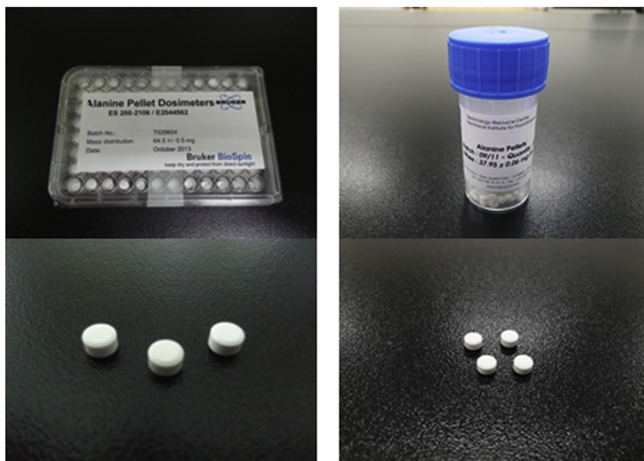
Fig. 1. The alanine dosimeter samples used in this intercomparison exercise (left: Bruker alanine dosimeter; right: Magnettech alanine dosimeter).
