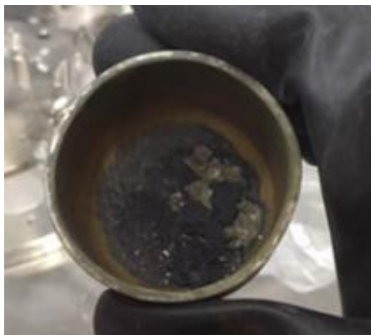
Fig. 11. The collected product after the salt distillation operation in Run #4.
