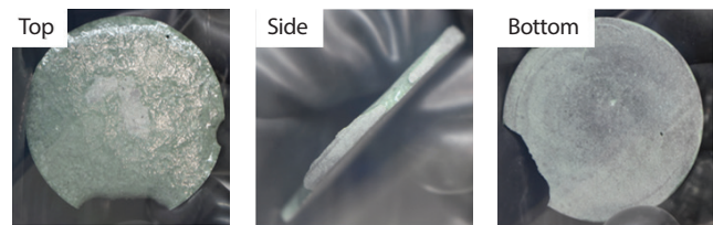
Fig. 8. Frozen rare earth chloride salt puck that was deposited underneath the tantalum crucible during the 13 days of ceramic and salt mixture interaction.
