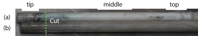
Fig. 3. Ceramic tube alumina-above (a) and mullite-below (b) after immersion in YCl_3 - SmCl_3 - NdCl_3 - PrCl_3 - CeCl_3 in LiCl-KCl at 773 K.
