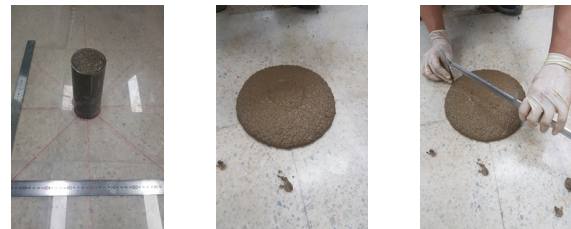
Fig. 3. View of flow test (ASTM D 6103, 2004)
