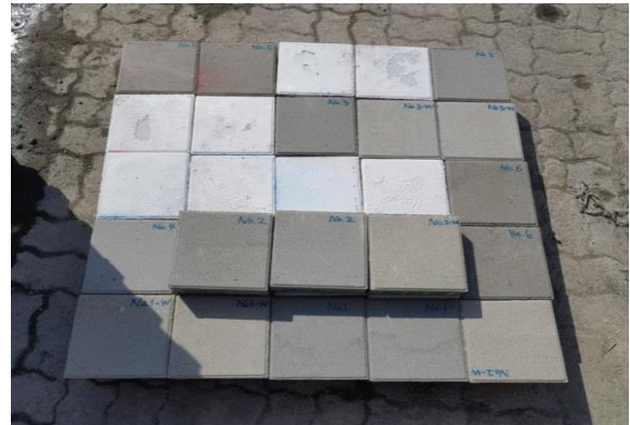
Fig. 4 Air purification concrete blocks specimens
