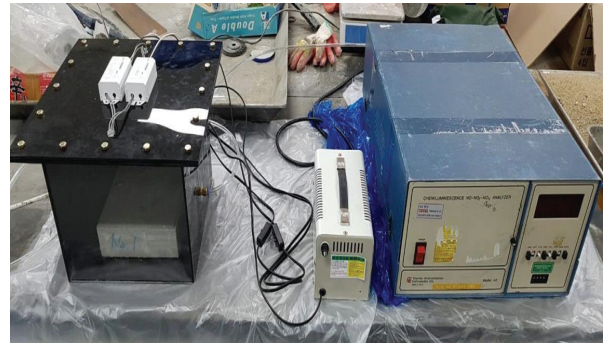
Fig. 6 Photograph of the test set-up for nitrogen oxide (NO x ) removal
