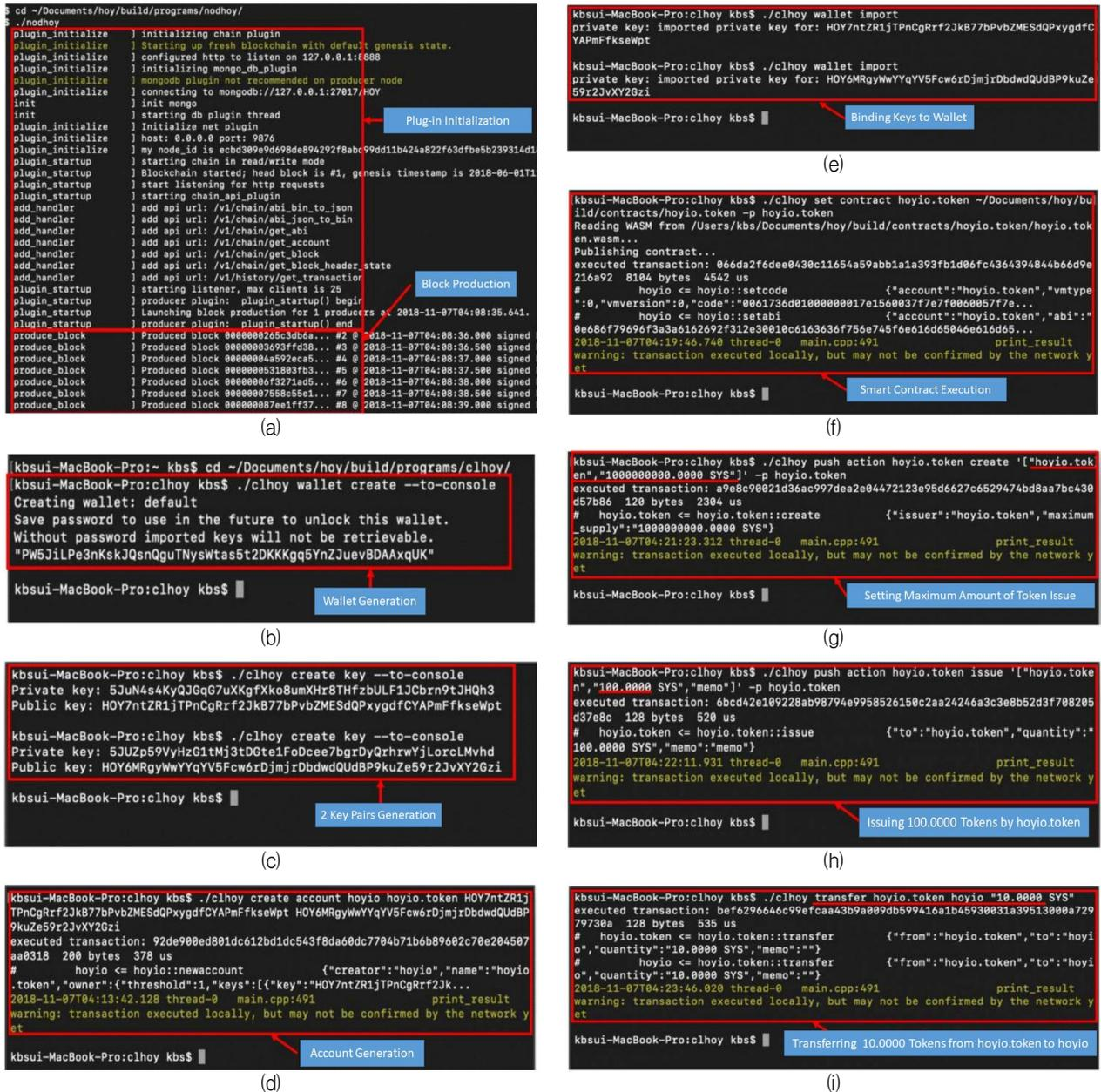
Fig. 2. Operation of “Q-Bone” blockchain platform : (a) Block production, (b) Wallet generation, (c) Key pairs generation, (d) Account generation, (e) Binding keys to wallet, (f) Smart contract execution, (g) Setting maximum amount of token issue, (h) Token Issuing, (i) Token Transferring.
