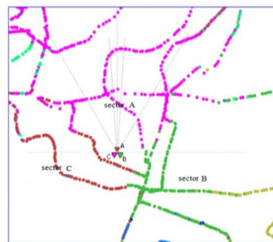
Fig. 10. Crossed Transmit Feeders.
