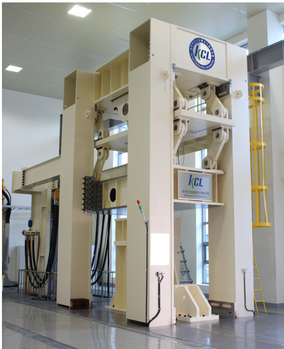
〈Fig. 5〉 Seismic control devices testing & evaluation system
