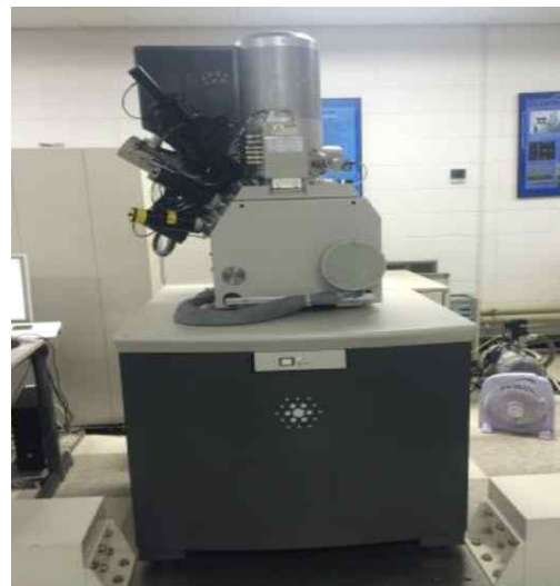
Fig. 1 Photograph of focused ion beam system (FEI, NOVA 600 Nanolab)
