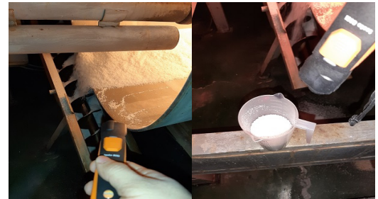
Fig. 2. Measuring temperature of the dried solar salt.
