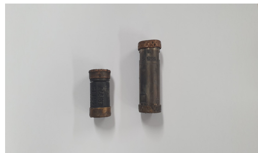
Fig. 2. Crusher gauge(left) vs. Piezo gauge (right)
