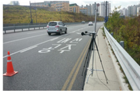
Fig. 3. Measuring noise level at the roadside
