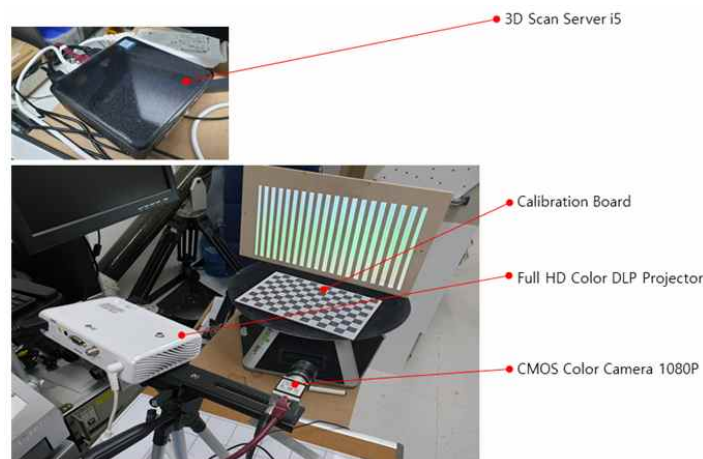
Figure 9. 3D Scanner system produced as a result of research
