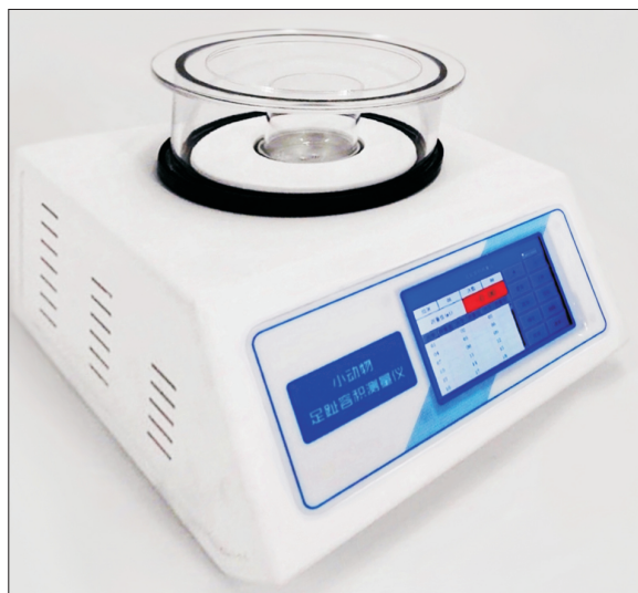
Fig. 1. The paw volume meter in this study. Paw volume meter: KW-7C, Nanjing Calvin Biotechnology Co., Ltd, Nanjing, Jiangsu, China.
