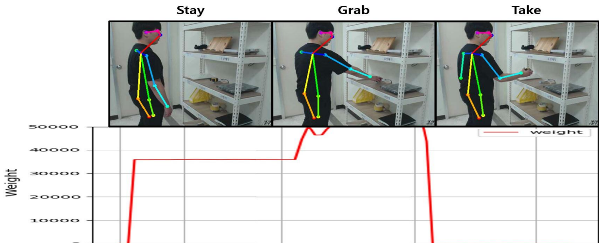
Fig. 7. Changes of the experimenter's behavior and the value of the load sensor according to the behavior
