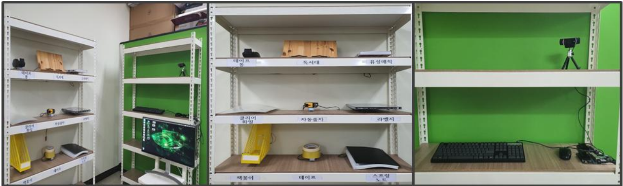
Fig. 5. Mock store view(left), Office supplies on the load sensor(middle), Jetson Nano board and webcam as server(right)
