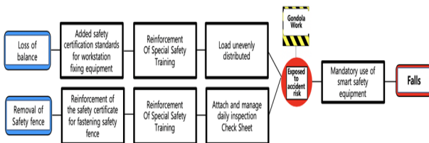
Fig. 7. Diagram of bow-tie risk assessment for removal of safety fence and human balance failure.
