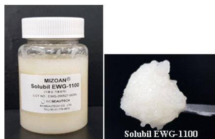
Fig. 2. Pictures of Solubil EWG-1100: INCI name is polyglyceryl-10 isostearate and polyglyceryl-10 oleate mixtures.
