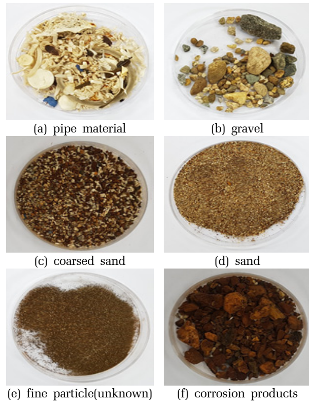
Fig. 4. Suspended solids discharged after air scouring.
