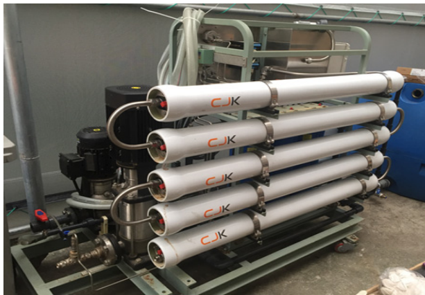
Fig. 3. Photograph of pilot scale RO system.
