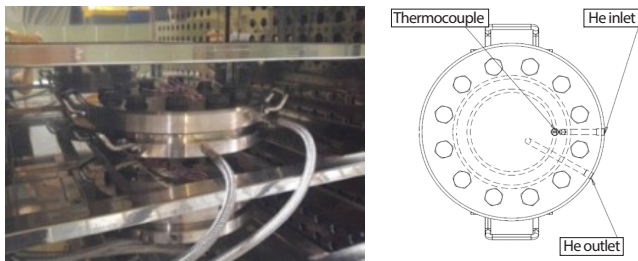
Fig. 5. Helium inlet and outlet of the flange assembly installed in chamber.
