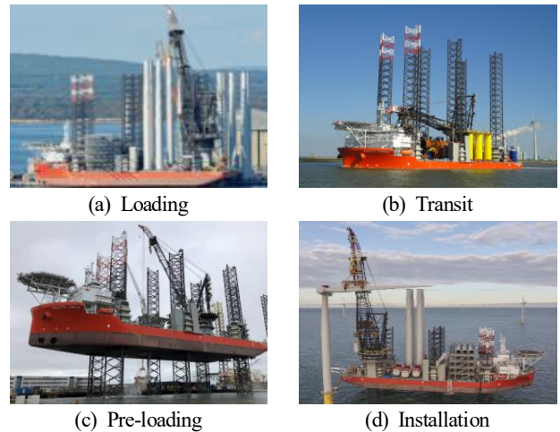
Fig. 2. WTIV operating process ( https://www.google.com , key word: SPO WTIV).
