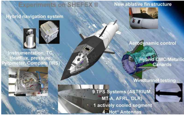
Fig. 23. SHEFEX II body and its components [56]
