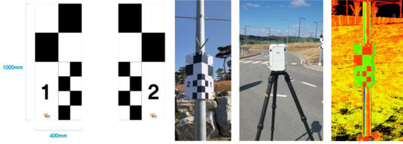
Fig. 3. Square type target (a) Design of the square type target plate; (b) Square type target plate on the pole; (c) LiDAR survey of the square type target plate; (d) Point cloud of the square type target plate
