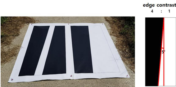
Fig. 2. Slanted edge target
