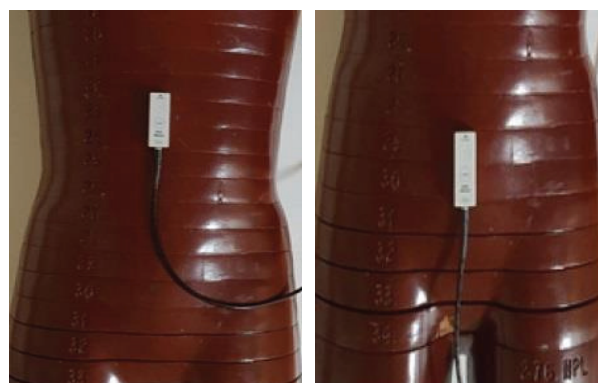
Fig. 4. Phantom and dosimeter were arranged in the center of the detector.
