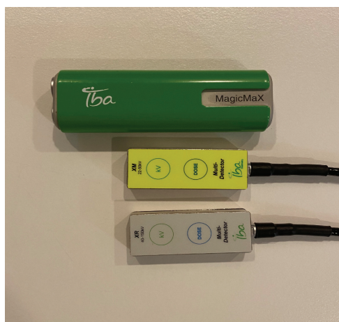
Fig. 3. The MagicMax Universal dosimeter was used in examination.
