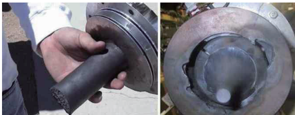
Fig. 4 Structural Failure of the Aerospike Nozzle [2,3]
