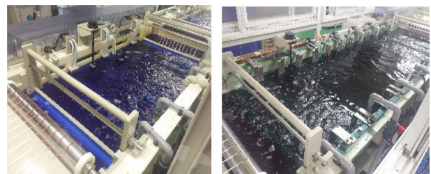
Fig. 1. Metal coating cylinder system: (a) Cu and (b) Ni coating system
