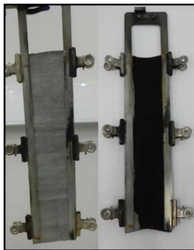
Fig. 8. Washed cotton ES/APP/f-GO (a) before and (b) after ASTM D6413
