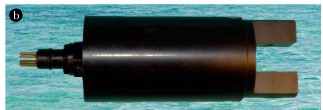
Fig. 2. (a) CTD device, (b) Sea point fluorometer sensor mounted on the CTD device.
