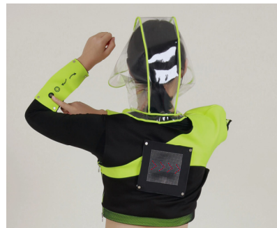
Fig. 11. Fabric Capacitive touch sensor
