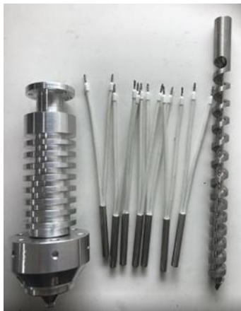
Figure 19. Screw, heat rod, barrel, nozzle of the smart head
