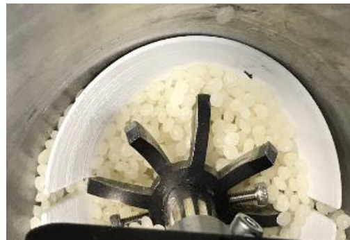
Figure 17. Grinding inside the hopper at the top of the smart head
