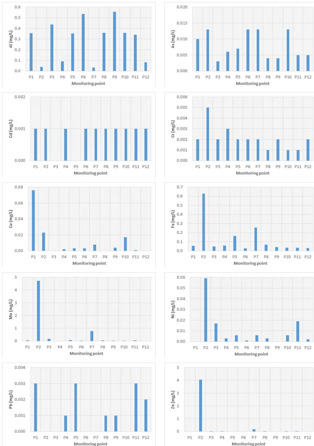
Fig. 4. Analysis results of heavy metals in the final effluent of wastewater treatment facilities.
