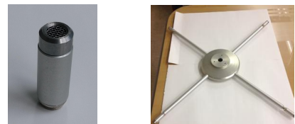
Fig. 7. Microphone sensor & 4 array sensor module
