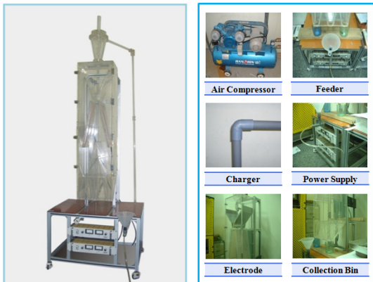
Fig. 7. Electrostatic separator for waste plastics by friction electric charge 21) .
