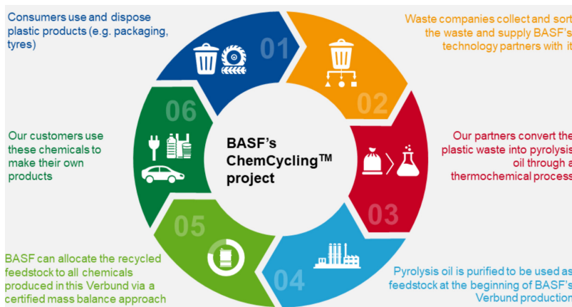
Fig. 2. BASF Chemical recycling of plastics waste 11) .
