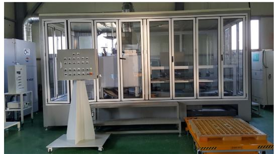
**Fig. 6.** Overview of heating separation apparatus of tempered glass.
