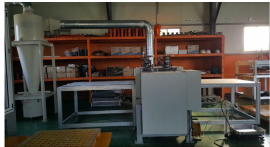
**Fig. 5.** Overview if roll crushing apparatus of tempered glass.
