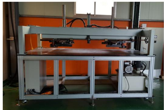
**Fig. 4.** Overview of separation apparatus of aluminum frame for ELP cell module.
