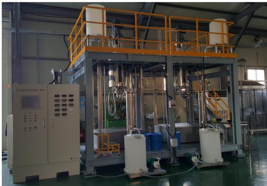
**Fig. 8.** Overview of leaching & precipitation reactor of ELP module.
