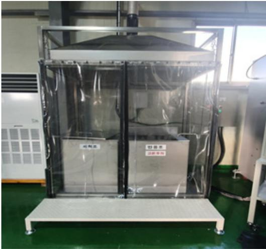
**Fig. 7.** Overview of swelling separation apparatus of back sheet component.
