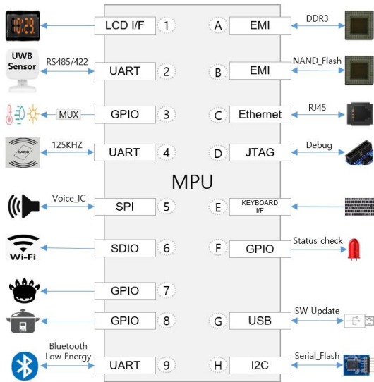
Fig. 4. Internal Configuration Diagram of IoT Gateway
